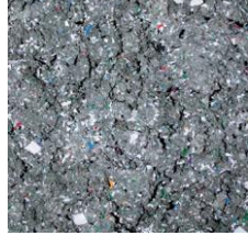
Screening waste from paper mills
