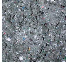
Screening waste from paper mills
